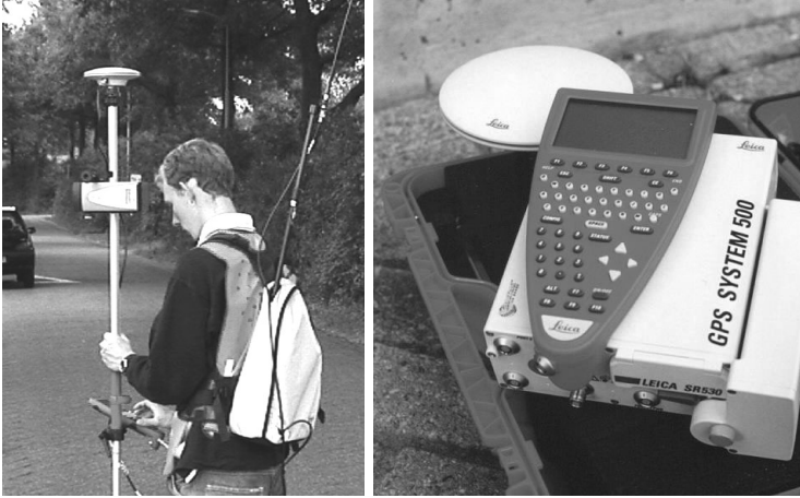
Figure 8. Real-Time Kinematic (RTK) GPS surveying: the surveyor directly ‘digitizes’ the points of interest in the field, by holding the antenna accurately in place for just a few seconds
